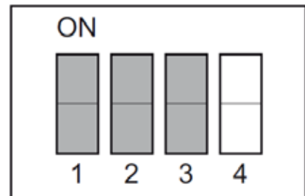
GREY dip-switches: total / partial Muting selection WHITE dip-switches: manual / auto. Restart selection Table 4: DIP-SWITCH SELECTION
